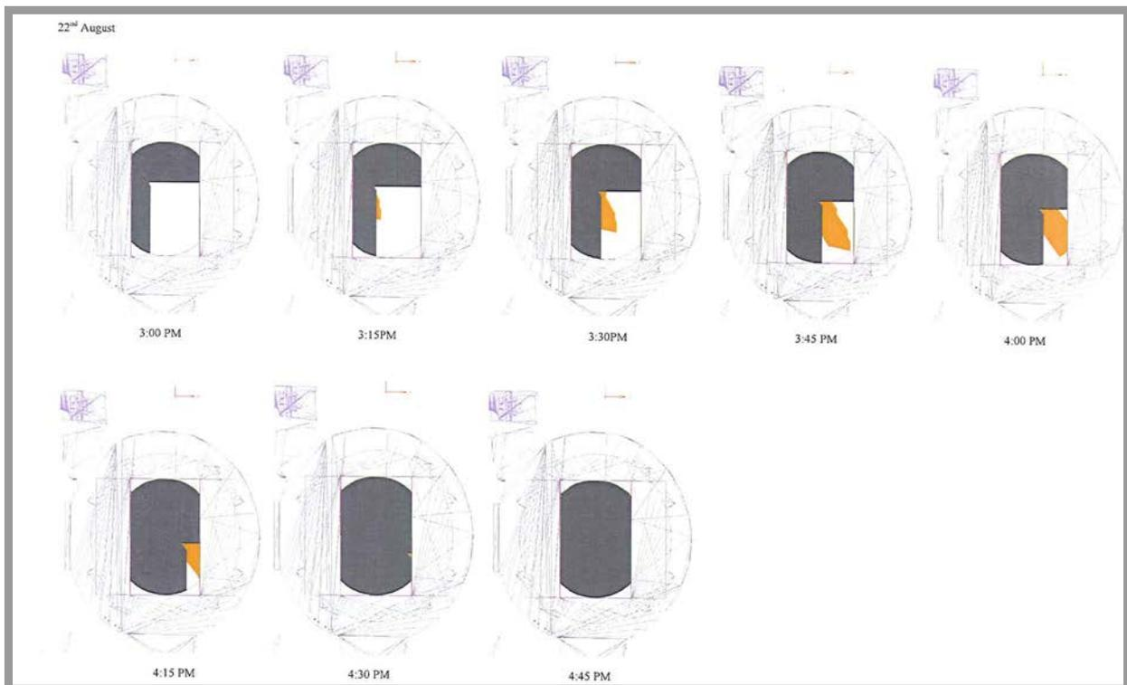
**Diagram 2: Shadow diagrams for additional overshadowing (shown in orange) caused by the proposal on 22<sup>nd</sup> August.**
