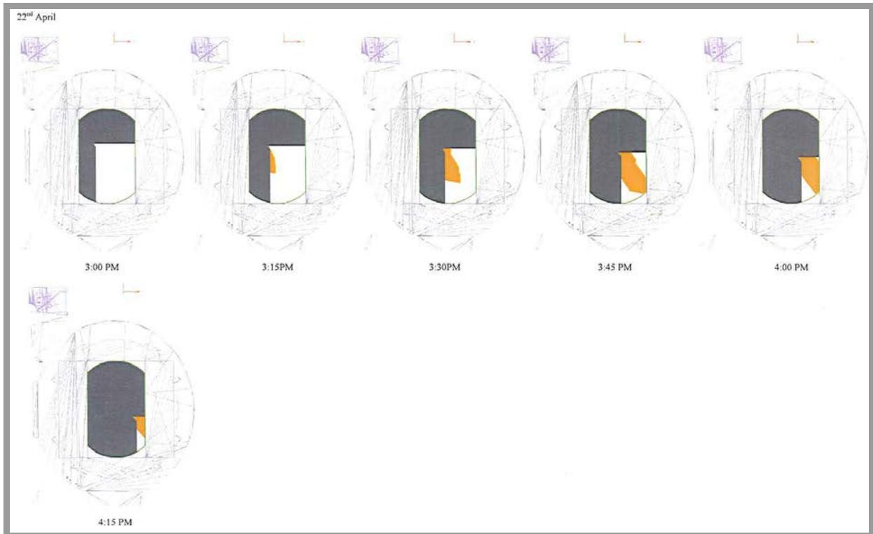
**Diagram 1: Shadow diagrams for additional overshadowing (shown in orange) caused by the proposal on 22<sup>nd</sup> April.**
